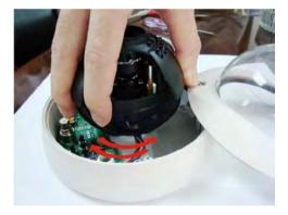
8. Twist the top to change the left/right angle of the lens
